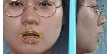
Figure 2: Tracking FAP values for Chinese visemes from both frontal and side views in a video recording (source: [6]).
